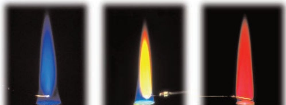
Figure 3 When an element is heated in a flame, it produces only certain colours or energies of light. Each element has its own unique line spectrum.
